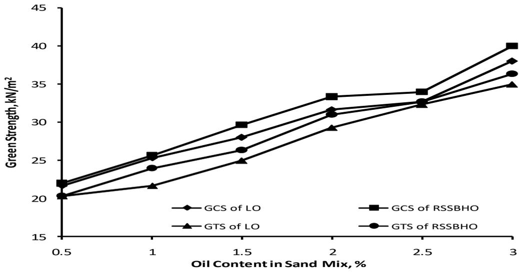
Figure 1: relationship between green strength of the core and oil content in sand mix
