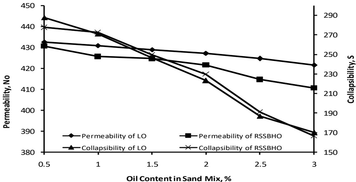
Figure 3: effect of oil content in sand mix on the permeability and collapsibility of the core
