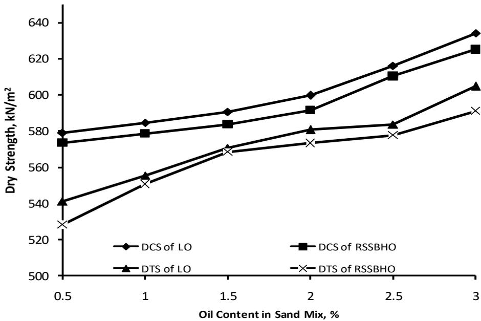
Figure 2: variation in dry strength of the core versus oil content in sand mix
