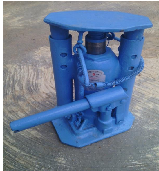
Figure 8: Modified hydraulic jack
