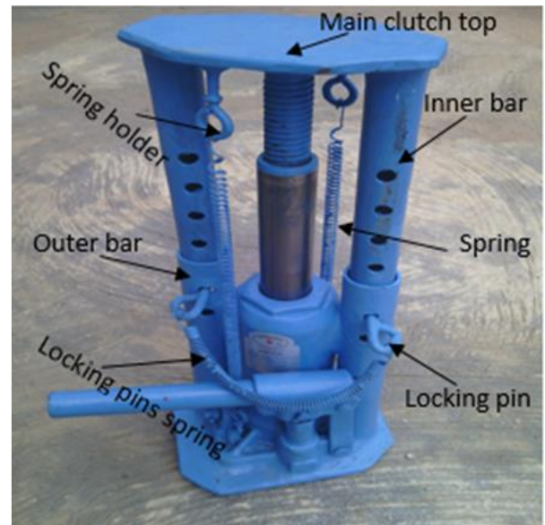
Figure 9: Modified hydraulic jack in use
