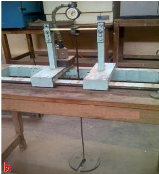
Figure 3 Testing Machines:- (a) Tensile test; (b) Bend test
