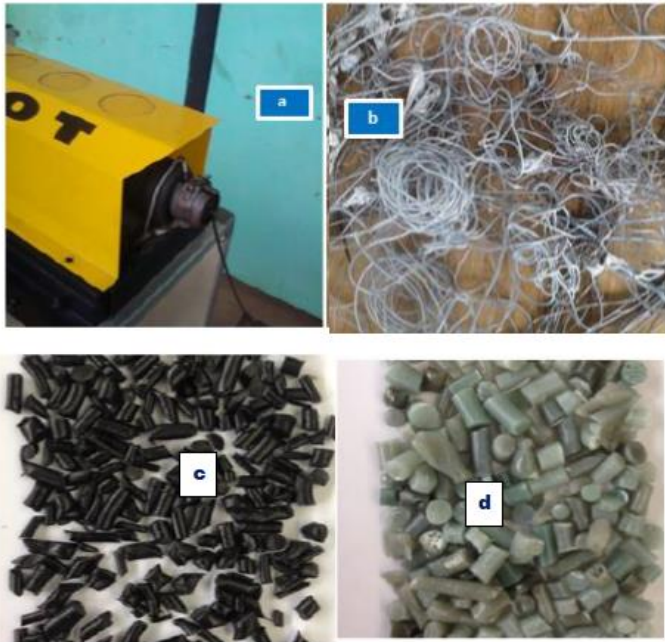
Figure 3: Output of the extrusion process: (a) molten extrudate (b) solidified extrudate (c) and (d) pelletized extrudate.
