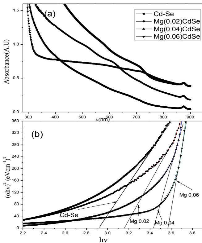
Figure 2(a) Plot of absorbance versus wavelength (nm), (b) Plot of  $(\alpha hv)^2$  vs  $h\nu$  for pure and Mg doped Cd-Se (0.02, 0.04 and 0.06 mole).
