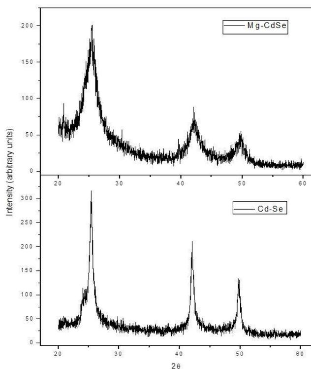
**Figure 1 XRD patterns of Cd-Se and Mg-doped (0.02 mole) Cd-Se QDs.**
