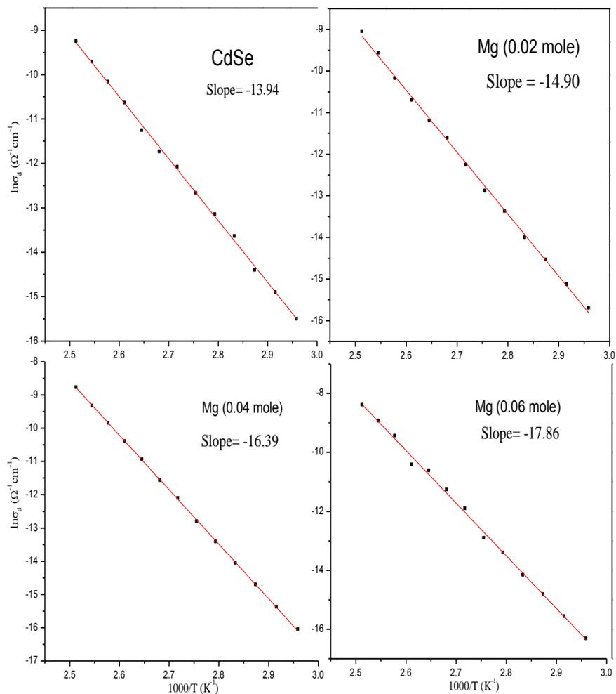
Figure 3 Temperature dependence of dark conductivity for pure and Mg doped Cd-Se (0.02, 0.04 and 0.06 mole).
