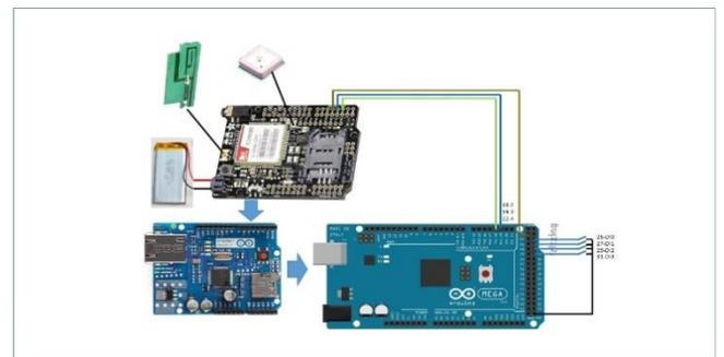
Figure 2: Block diagram of the GSM/GPS-based Vehicle Tracking System
