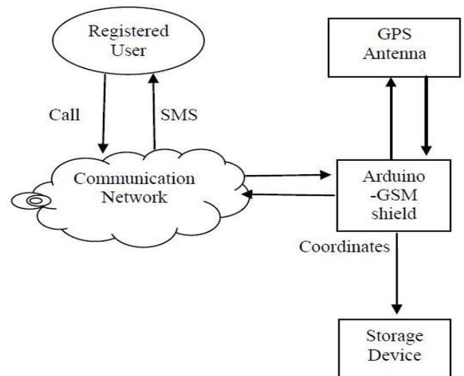
Figure 1: Architecture of Real-time GPS tracking system
