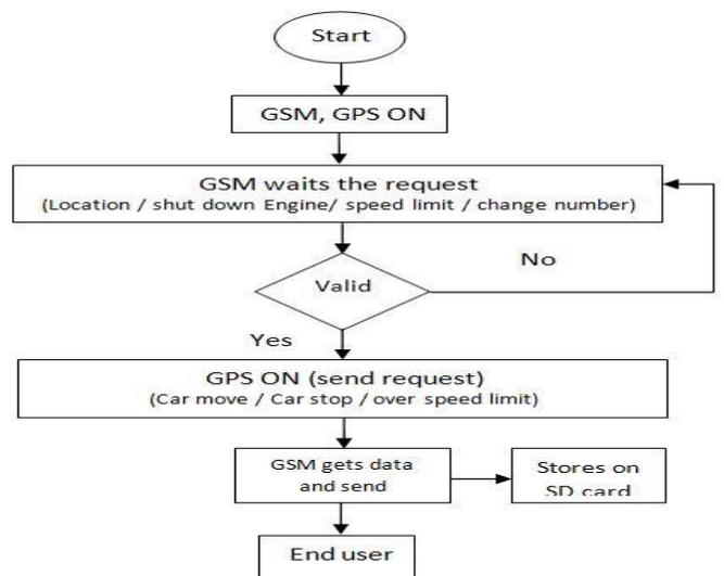
Figure 5: Flow chart GPS tracking system
