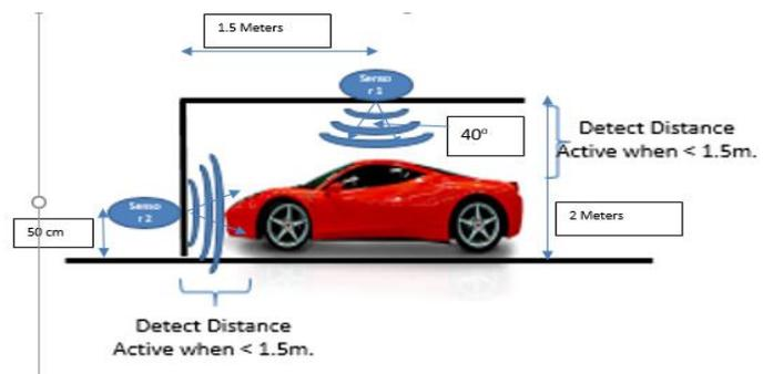
**Figure 4: Sensor Installation**
