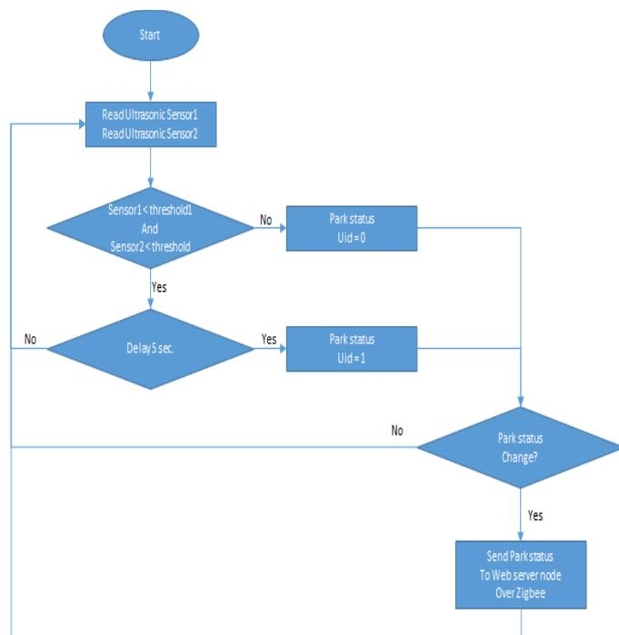
Figure 5: Sensor node circuit flow chart
