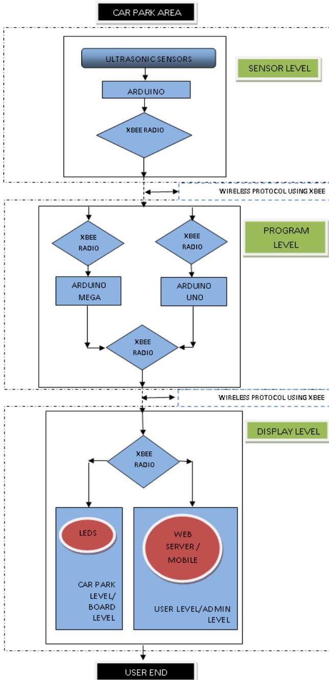
**Figure 2: System Architecture of smart car park.**
