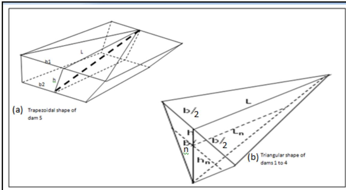
**Figure 2: Approximate dam wall cross sections used to calculate actual runoff in the reservoir**
