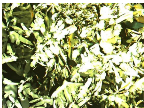
Fig.2. Photomicrograph of the texture observed on cooling from the isotropic state for A-8 at 214.5°C.
