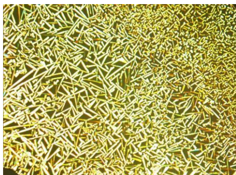
Fig.1. Photomicrograph of the texture observed on cooling from the isotropic state for A-10 at 210°C.
