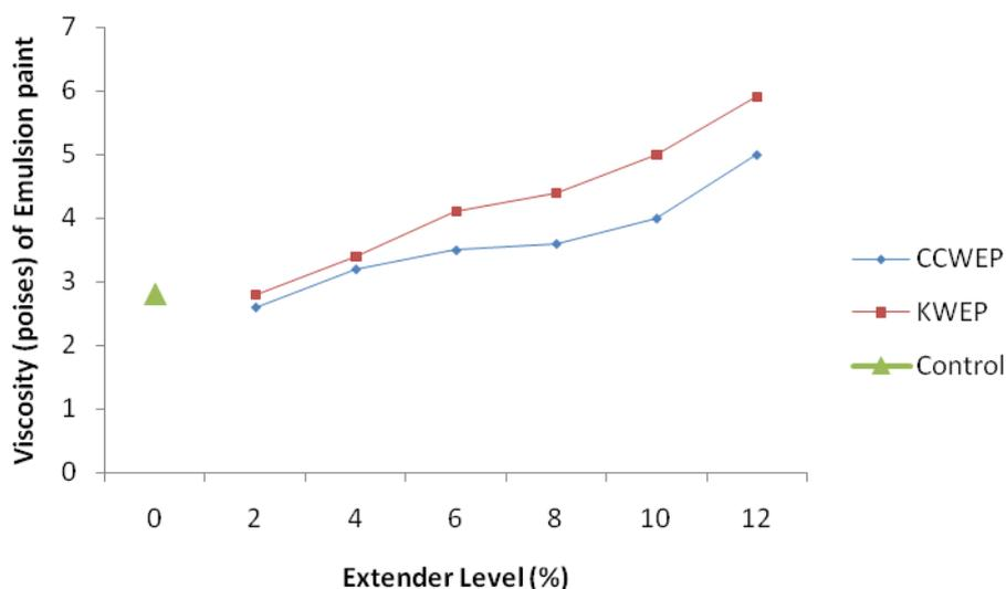
Fig. 4 Plots of Viscosity (poises) of emulsion paint versus extender Level
