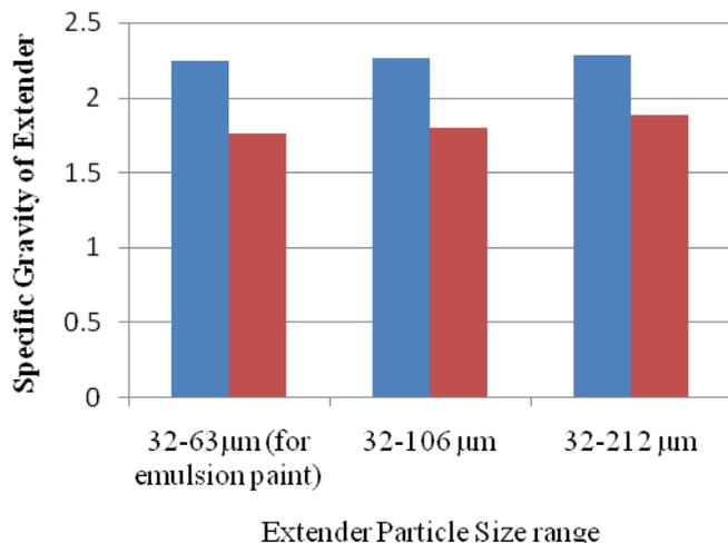
**Fig.1 Plot of specific gravity of extender against emulsion type**
