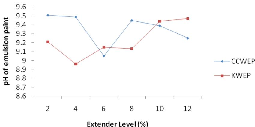
**Fig.2 Plots of pH values of Emulsion paints versus extender level**
