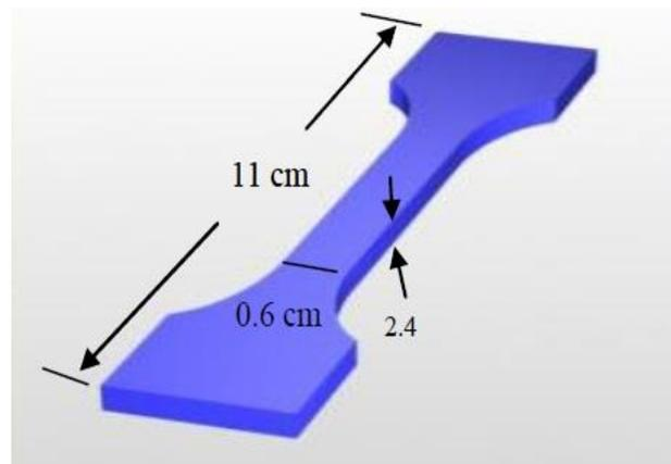
Figure (2) tensile specimen coupon dimensions centimeters.
