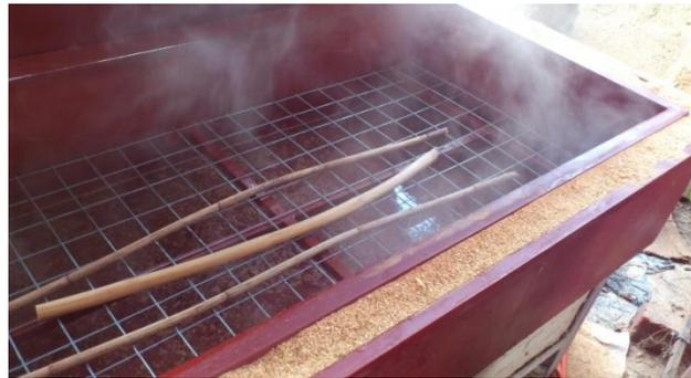
Fig 2 Samples of rattan on galvanised metal mesh rack
