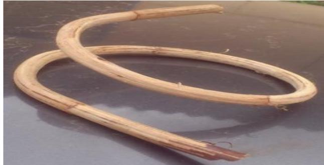
Fig 4 Test result of steam bending
