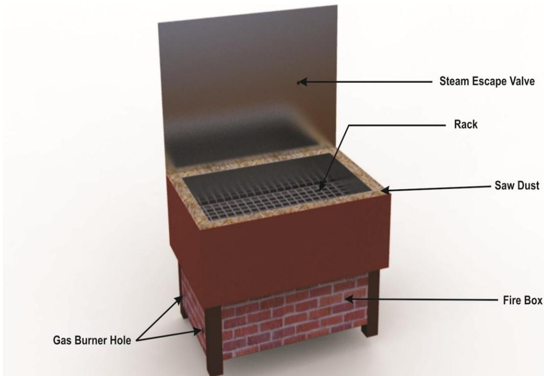
Fig 1 A. Rhino representation of the gas fired steamer tub.
