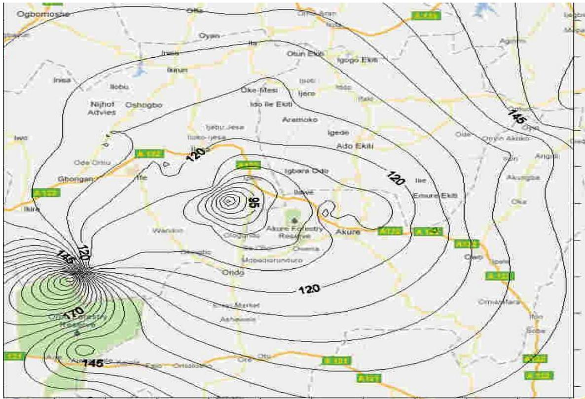
Fig. 4: Map of Coverage area shown contour of transmission loss (dB)
