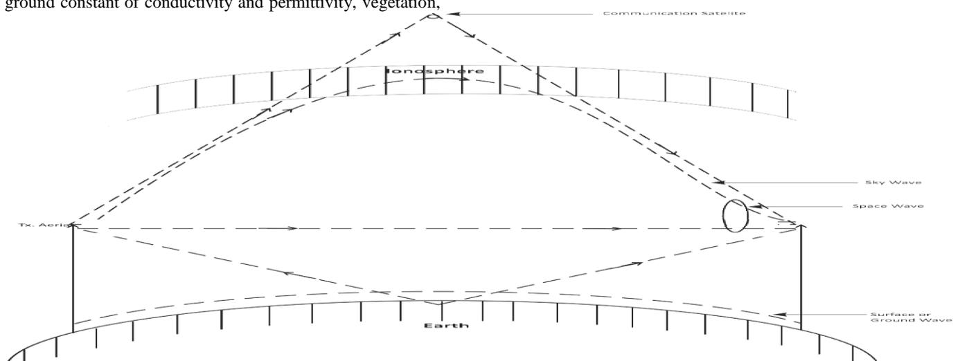
Fig. 1: Modes of Wave Propagation
