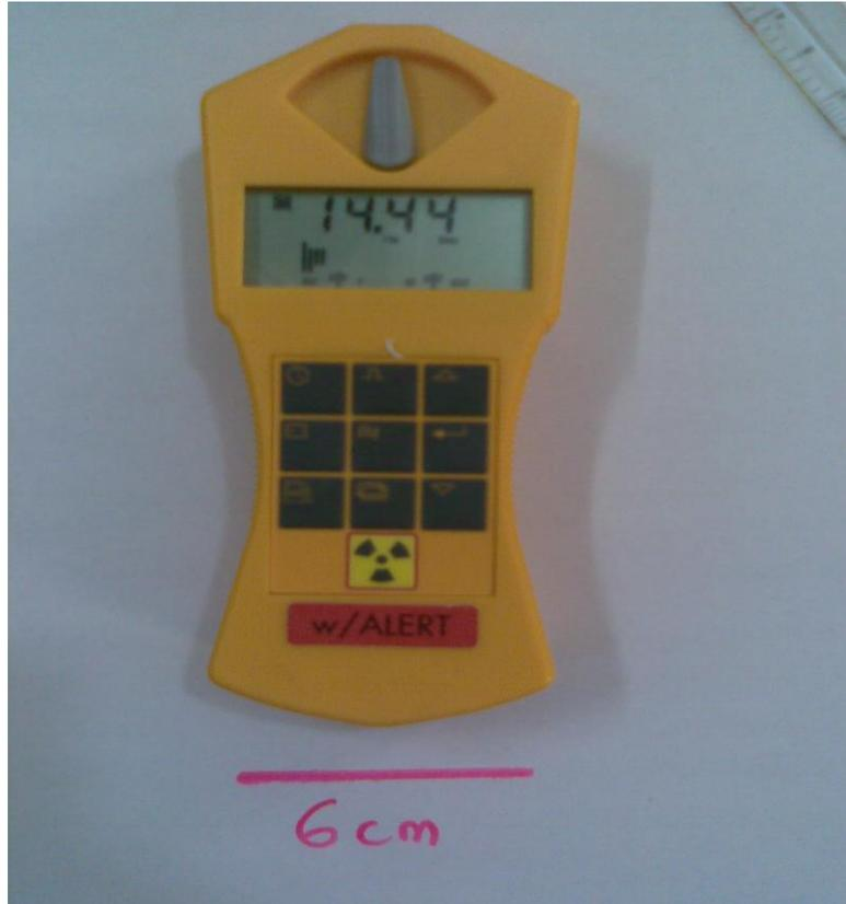
**Fig.7. Gamma Scout Instrument**
