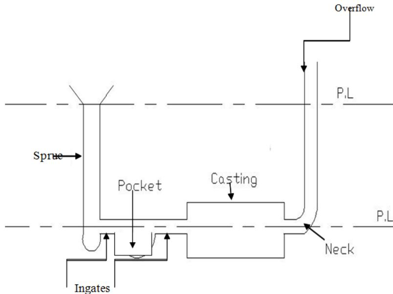
Figure 1: Schematic diagram of mould produced
