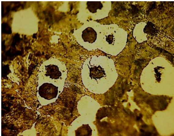
**Figure 2c:** Micrograph of as cast ductile Iron inoculated with 18g powdered graphite and 18g powdered ferrosilicon showing more ferrite around the nodules (bull's eye) in pearlite matrix (X800).=
