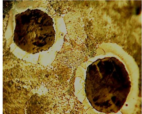
**Figure 2b:** Micrograph of as cast ductile iron inoculated with 36g powdered ferrosilicon mixed with 36g graphite showing ferrite ring around the nodules in pearlite matrix (X800)
