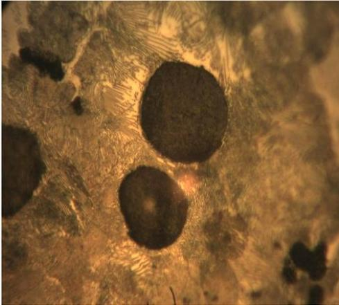
**Figure 2a:** Micrograph of as cast ductile iron inoculated with 72g powdered graphite showing nodules in pearlite matrix (X800)
