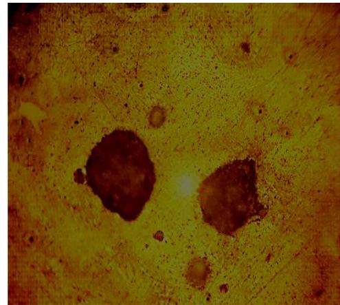
**Figure 2d:** Micrograph of as cast ductile iron inoculated with 72g powdered ferrosilicon showing nodules in entirely ferrite matrix (X800)
