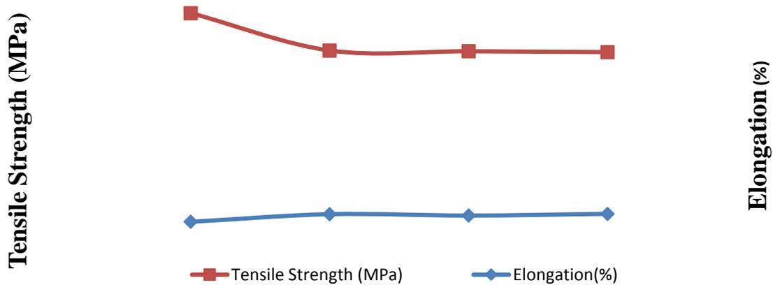
Figure 3: Plot of Tensile strength and Percentage Elongation of test samples against Inoculant addition
