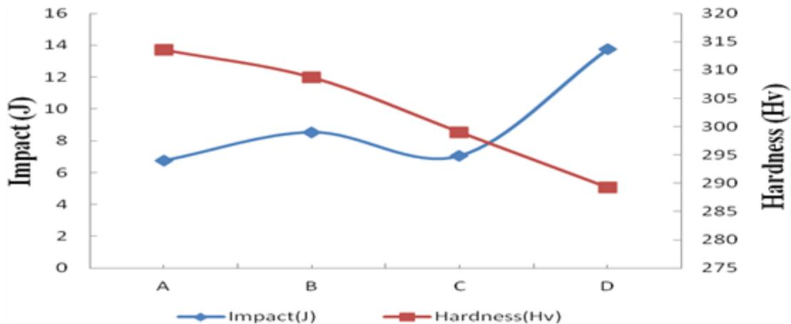
Figure4: Plot of Hardness and Impact energy against Inoculants addition
