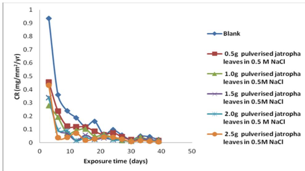
Fig.1: Plot of corrosion rates against exposure time for medium carbon steel immersed in 0.5M NaCl solution with and without pulverized *jatropha* leaves as inhibitor
