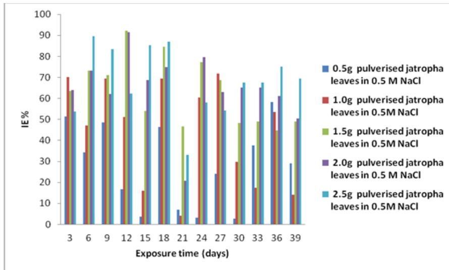
Fig. 2: Plot of inhibition efficiency against exposure time for medium carbon steel immersed in 0.5M NaCl solution with and without pulverized jatropha leaves as inhibitor
