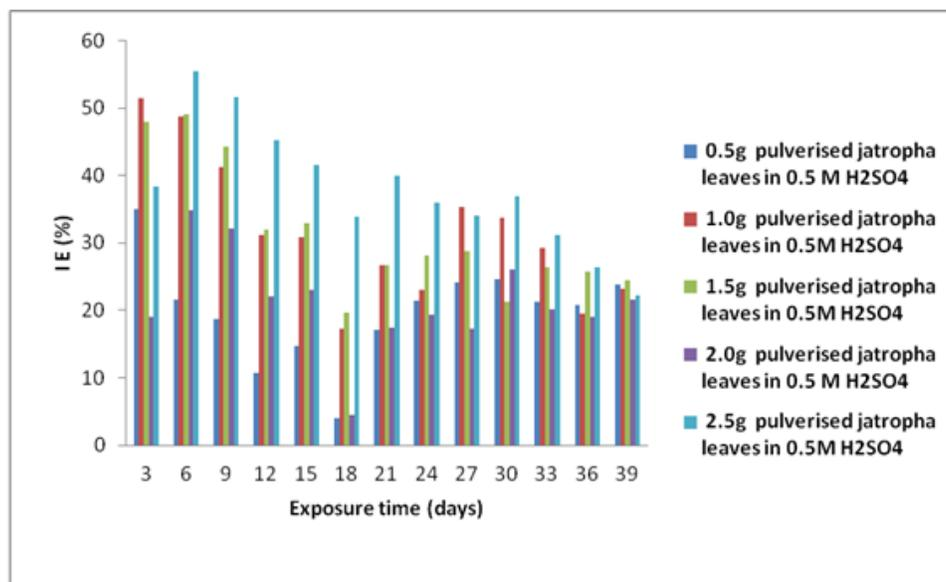
Fig. 4: Plot of inhibition efficiency against exposure time for medium carbon steel immersed in 0.5M H<sub>2</sub>SO<sub>4</sub> solution with and without pulverized jatropa leaves as inhibitor
