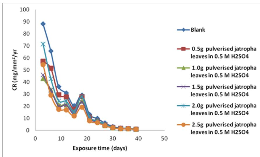
Fig. 3: Plot of corrosion rates against exposure time for medium carbon steel immersed in 0.5M H<sub>2</sub>SO<sub>4</sub> solution with and without pulverized jatropha leaves as inhibitor
