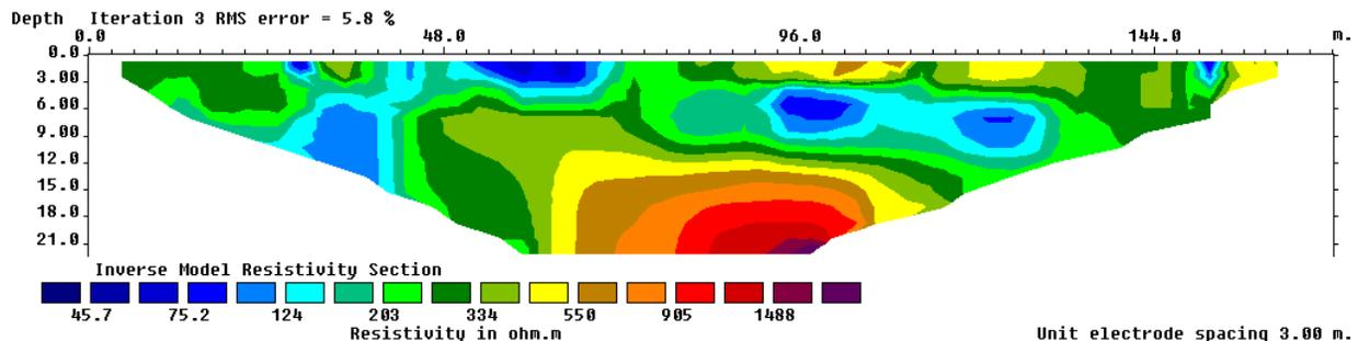
Fig. 5. 2D resistivity model along traverse B
