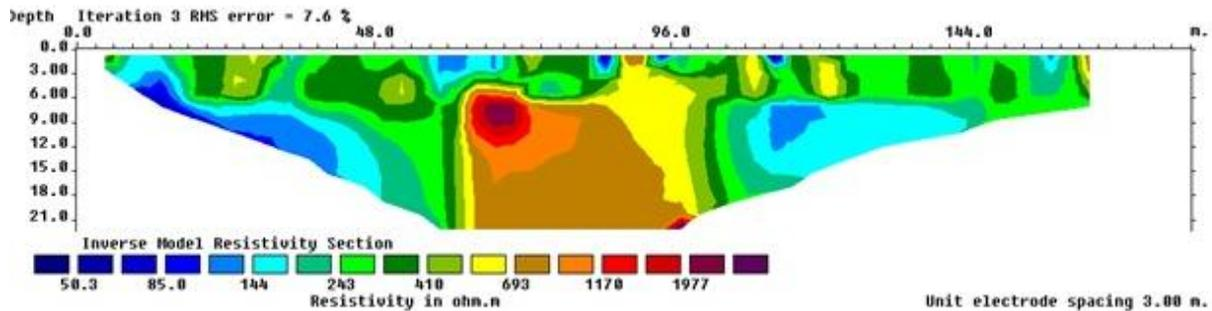
Fig. 4 2D resistivity model along traverse A
