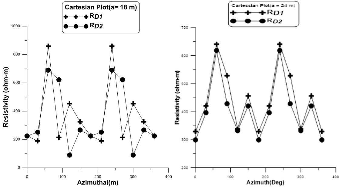
Fig.7b: Cartesian graphs of electrode spacing of a = 18 and 24 m along traverse C
