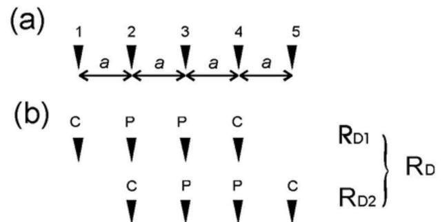
Figure 3. Offset Wenner electrode arrangement and resistance measurement.
