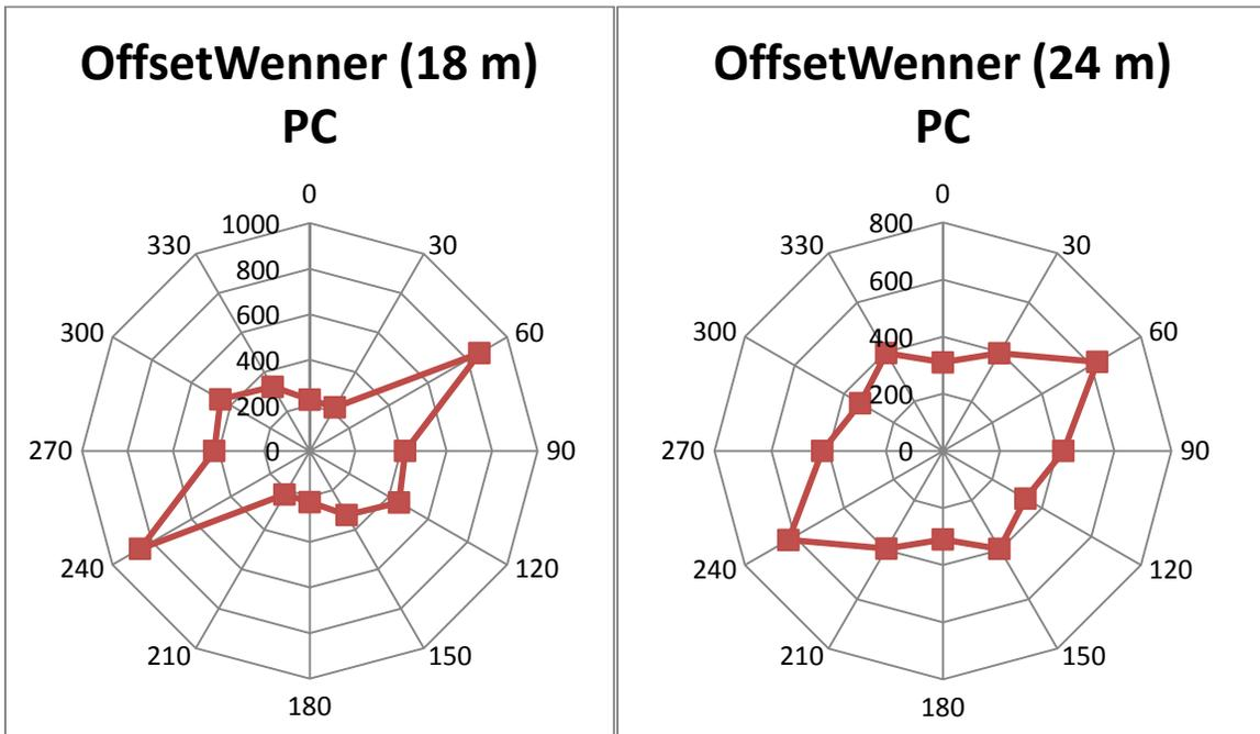
Figure. 7b: Offset Wenner sounding diagrams of azimuthal resistivity survey along traverse C
