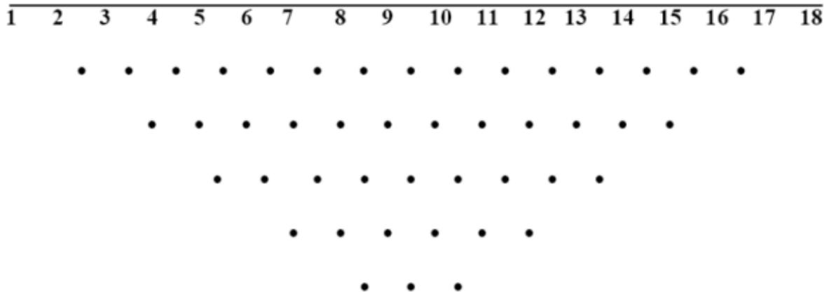
Figure 2. The arrangement of electrodes for a 2-D electrical survey and the sequence of measurements used to build up a pseudosection (After Aizebeokhai, 2010)
