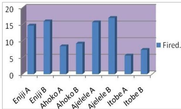
**Figure 2: Fired Modulus of Rupture of Selected Clays**
