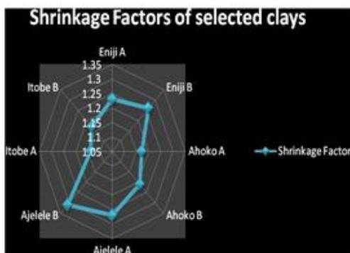
**Figure 1: Factors of Shrinkage of Selected Clays**
