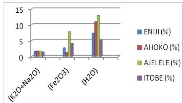
**Figure 3: Alkali oxides, Iron oxide and Water Percentages in Selected Clays**
