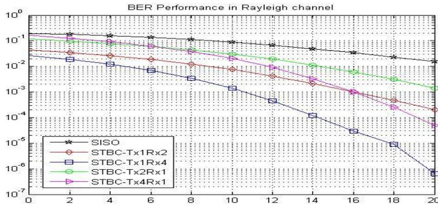
Fig 3 (b): Different number of Transmit and Receive Antenna in Rayleigh channel
