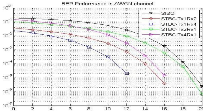
Fig 3(a): Different number of Transmit and Receive Antenna in AWGN channel
