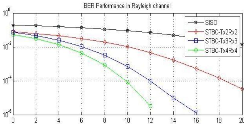
Fig 3(d): Same number of Transmit and Receive Antennas in Rayleigh channel
