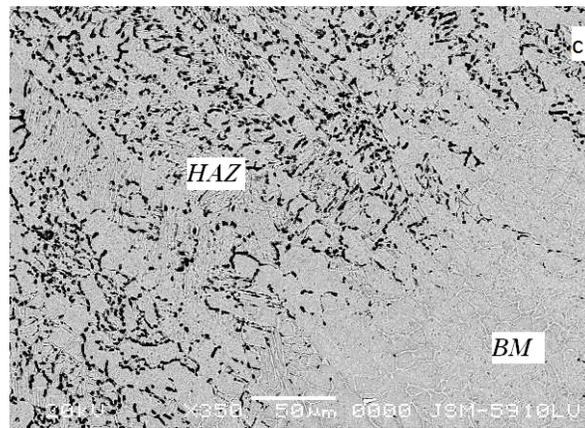
Fig. 5(a) Optical Micrographs of HAZ and WM (X200), (b) Stereo Micrographs of HAZ, WM and BM (X200), (c) SEM Micrographs of HAZ and BM (X350)
