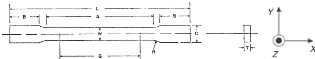
Fig.1. Test Specimen for the Tensile Test
