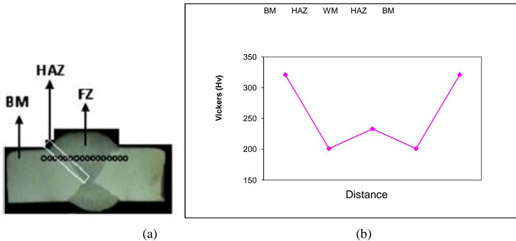
Fig. 3. Vickers Hardness, (a) Profile Scheme of the Hardness (b) Graphic of the Hardness Measured
