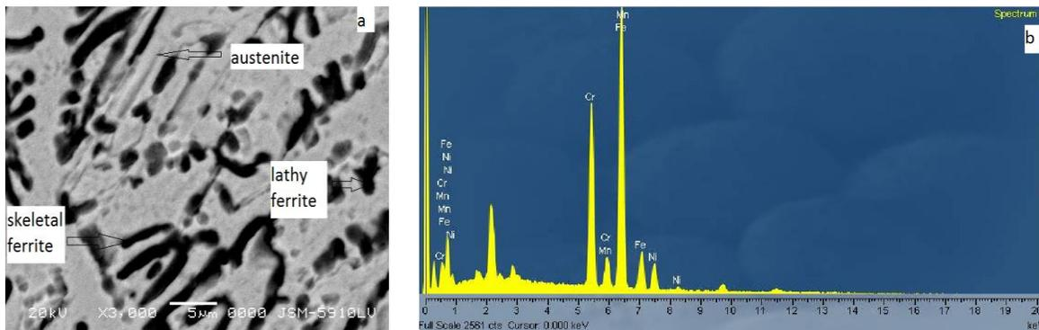
Fig. 6 SEM Micrographs and EDS Analysis of WM (X3000)
