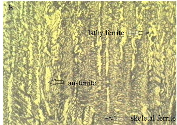
Fig. 4. Micrographs of the Microstructures, (a) BM (b) TIG Welding at the Fusion zone (X200)
