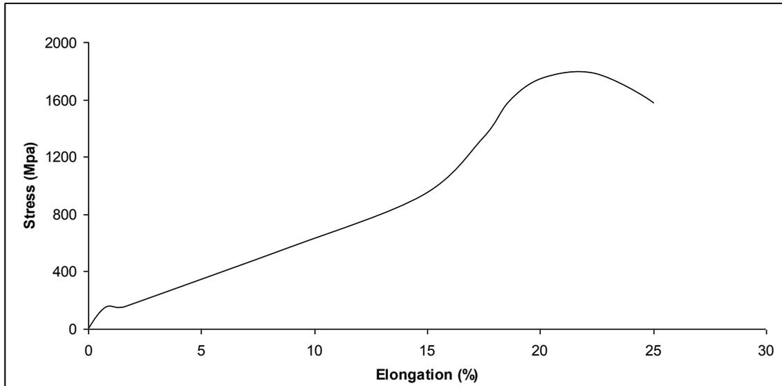
Fig. 2. Tensile Test Graphic of 304 SS Jointed by TIG Welding
