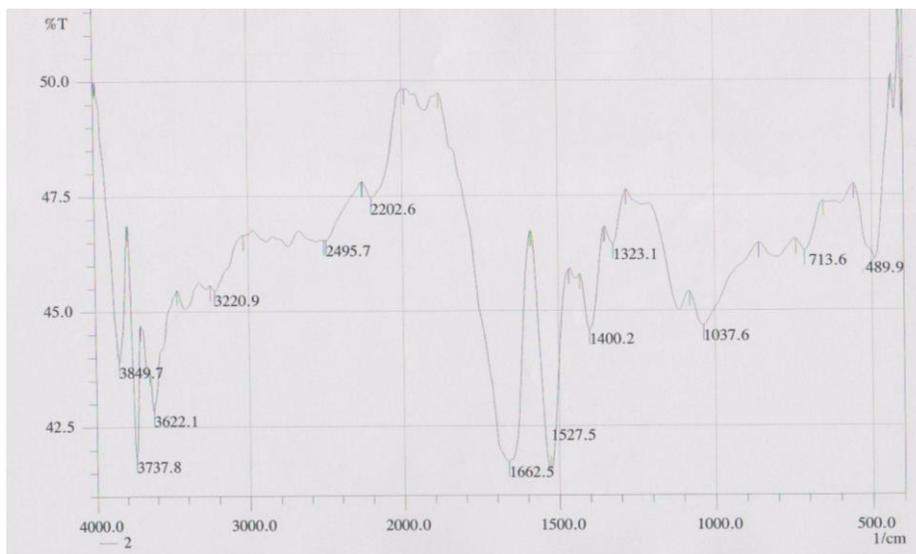
Fig. (10): FT-IR spectrum for Ca-alginate beads
