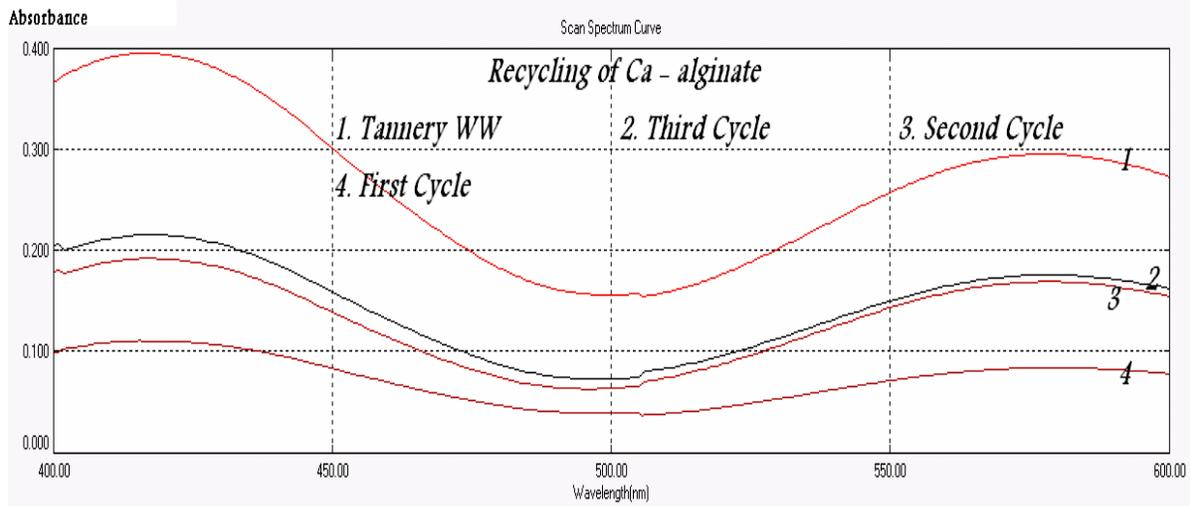
Fig. (4): Scan spectrum curve of tannery wastewater sample after recycling of Ca-alginate beads
