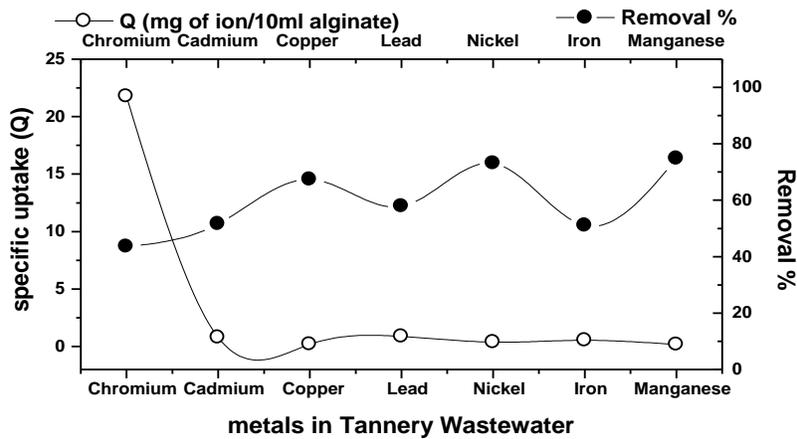
Fig. (3) Heavy metals adsorption capacities after treatment by Ca-alginate
