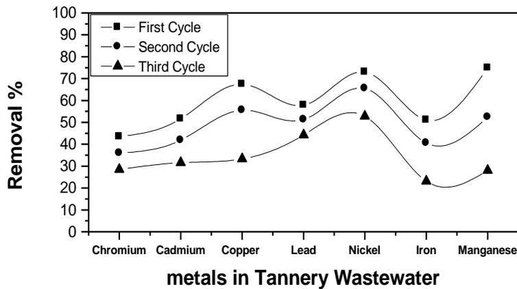
Fig. (6) Heavy metals adsorption capacity after recycling of ca-alginate beads
