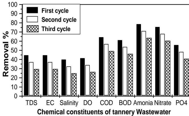
Fig. (5) Removal percentage of chemical constituents after recycling of Ca-alginate beads
