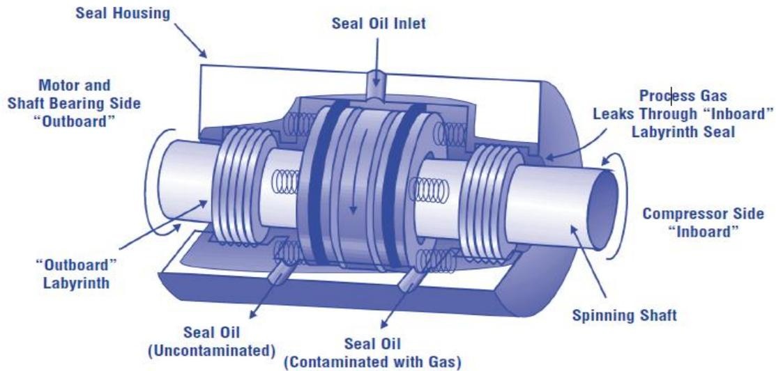
Fig 2: Diagram of a wet (oil) seal. (Courtesy of Natural Gas STAR partners, 2003)
