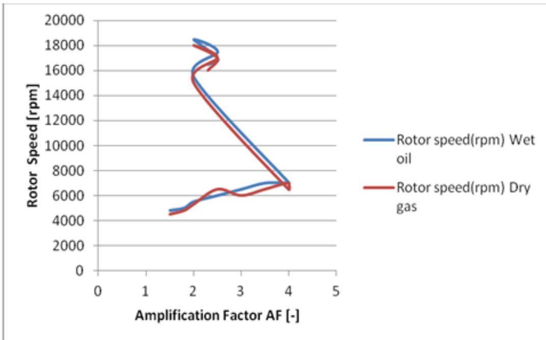
Fig 5: Chart showing Critical speed against Amplification factor for HP (BOG) compress
