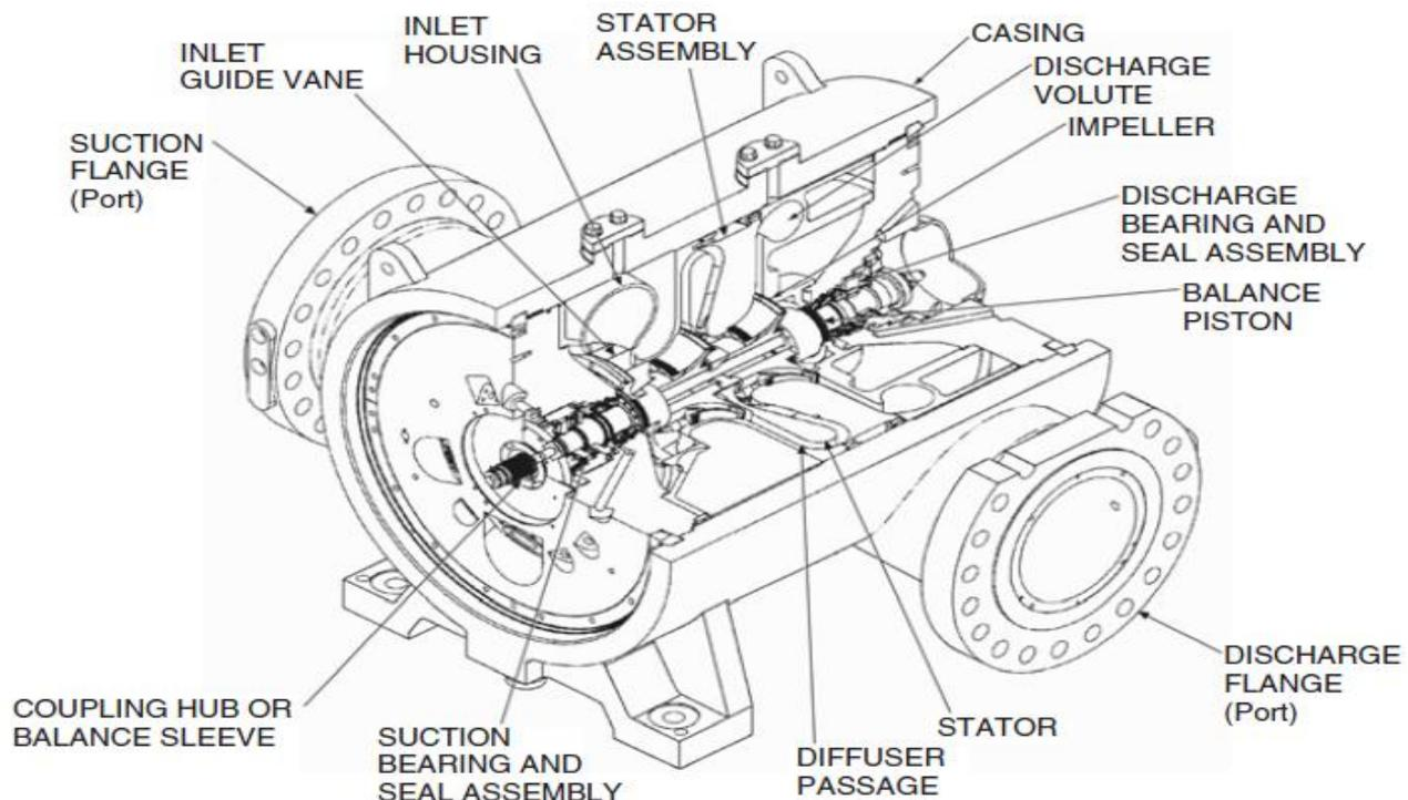
Fig 1: Typical centrifugal compressor cutaway, Courtesy GPSA, 2004
