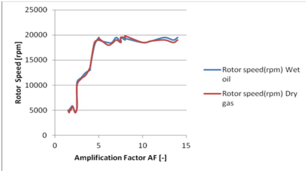
Fig 4: Chart showing Critical speed against Amplification factor for LP (BOG) compressor
