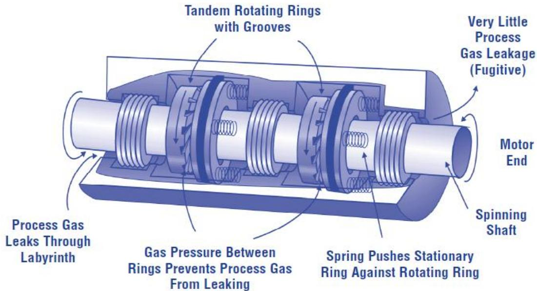
Fig 3: Diagram of a dry (gas) seal. (Courtesy of Natural Gas STAR partners, 2003)
