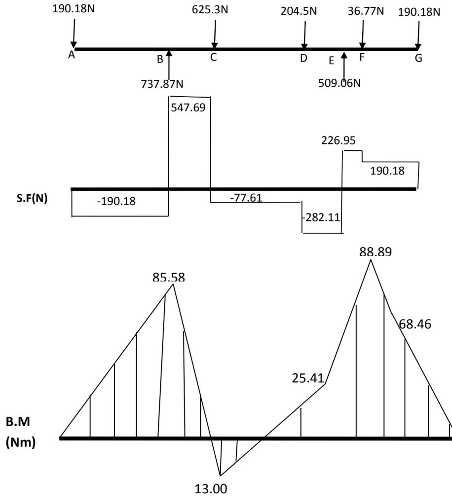
Figure 1b: The Line Diagram of Loads, Shearing Forces and Bending Moment Diagrams
