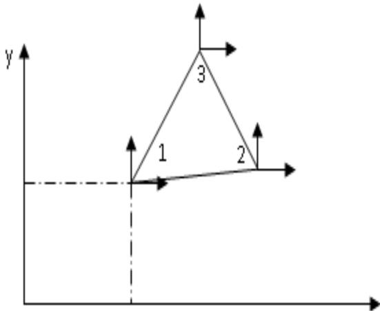
Figure 2: Local and Global Coordinates and Nodes of Nodal Forces and Displacements
