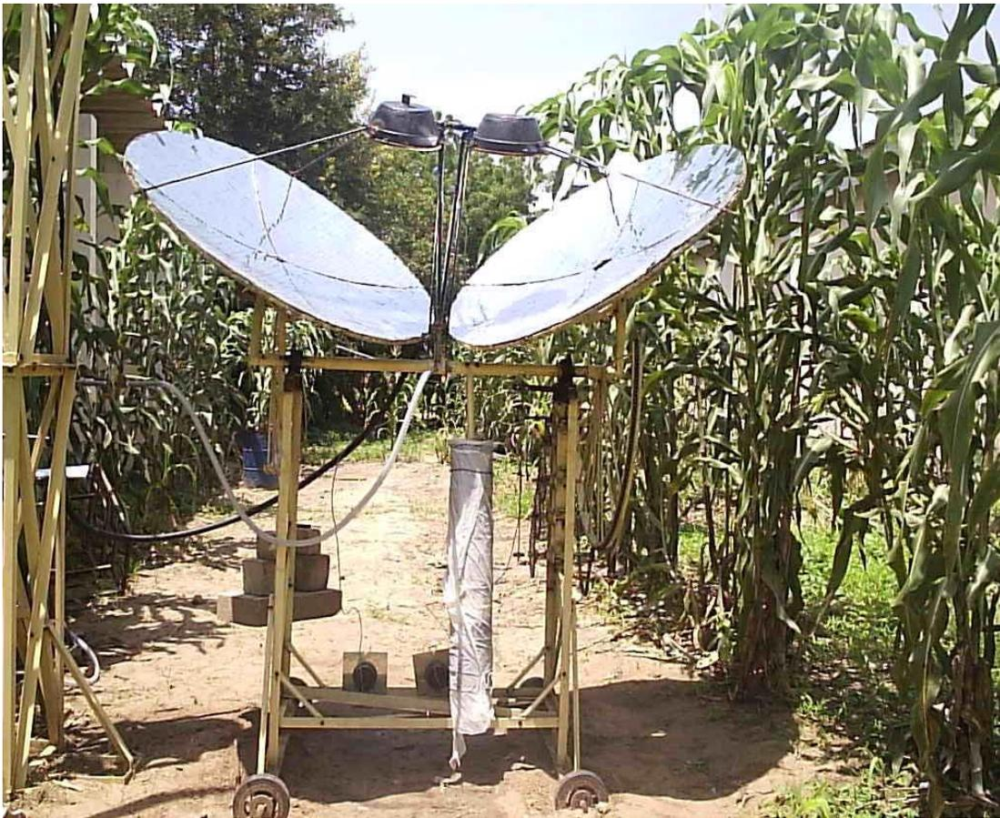
Figure 4: Support Structure of Solar Tracking Bi-Focal Collector System on Field Test.
