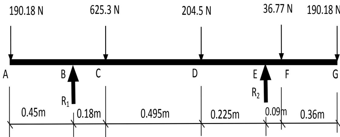
**Figure 1a : Various Loads acting on the Rotating Shaft Support**
