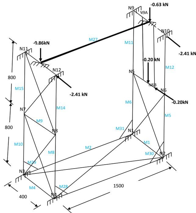
Figure 3: Geometry of the Structural Support
