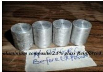
Plate 2: the Unexposed Specimens of the Composite as Prepared
