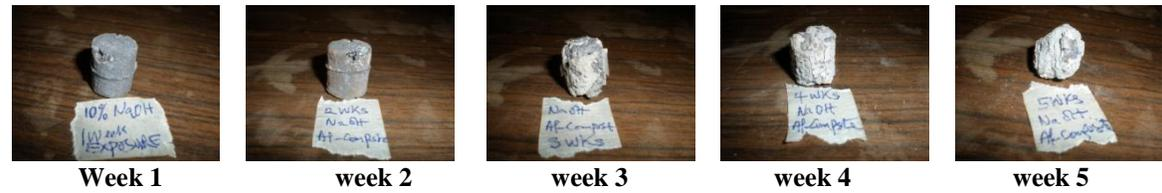
Plate 4: Specimens Evaluated in 10 Weight Percent NaOH Solution
