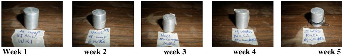
Plate 3: Specimens Evaluated in 5 Weight Percent NaCl Solution
