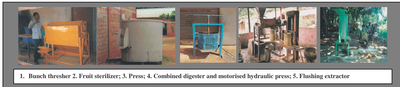
Plate 4 - Examples of improved/mechanized technology applied in palm oil extraction
