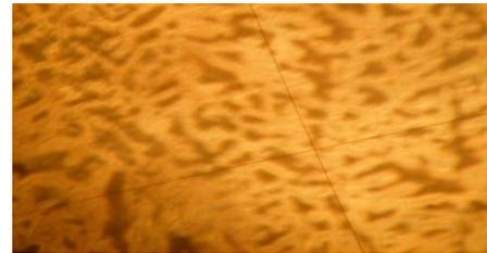
Plate 4: Sample 5 (2.5% glass particles), As-Cast showing dendritic solidification in the Matrix of the Aluminum. X200
