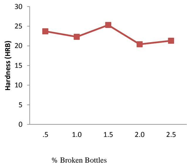
Figure 1: Variation of Hardness with Percentage Addition of Broken Bottles
