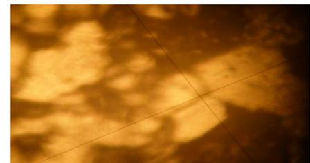
Plate 5: sample 3 (1.5% glass particles) showing the age hardened microstructure at 190°C for 5 hours. The black phase is the precipitate and the clear background represents the aluminum matrix. X200
