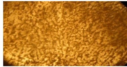
Plate 3: Sample 4 (2.0% glass particulates) As-Cast showing the second phase in dendritic solidification in the Matrix of the Aluminum. X 200
