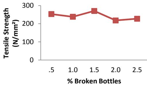
Figure 2: Variation of Tensile Strength with Percentage Addition of Broken Bottles
