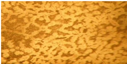
Plate1: Sample 1 (0.5% glass particulate) As-cast showing the second phase in dendritic solidification in the grains of the Aluminum. X200
