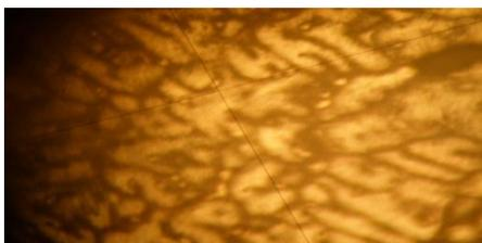
Plate 2: Sample 3 (1.5% glass particulate) As-Cast showing the particulates and dendrites in the Matrix of the Aluminum. X200
