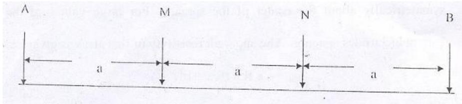
Figure 4: Wenner electrode array
