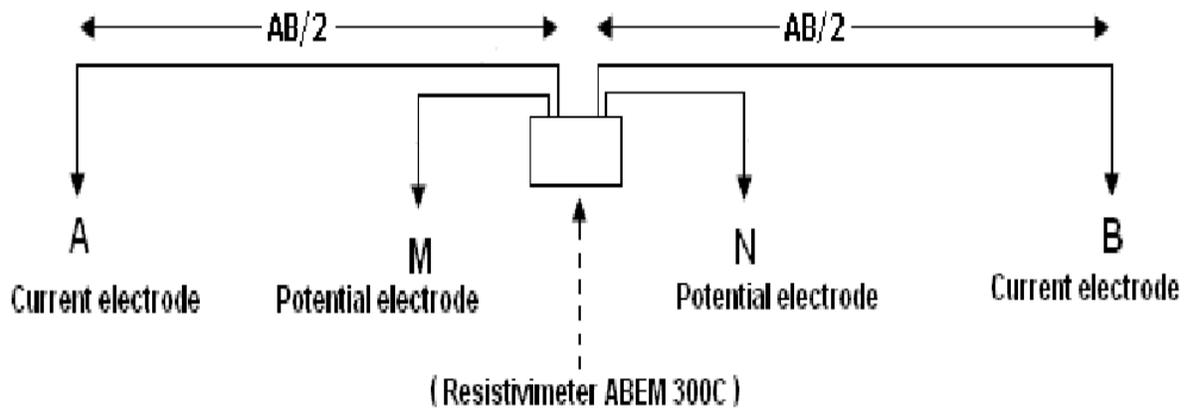
Figure 2: Schlumberger electrode array
