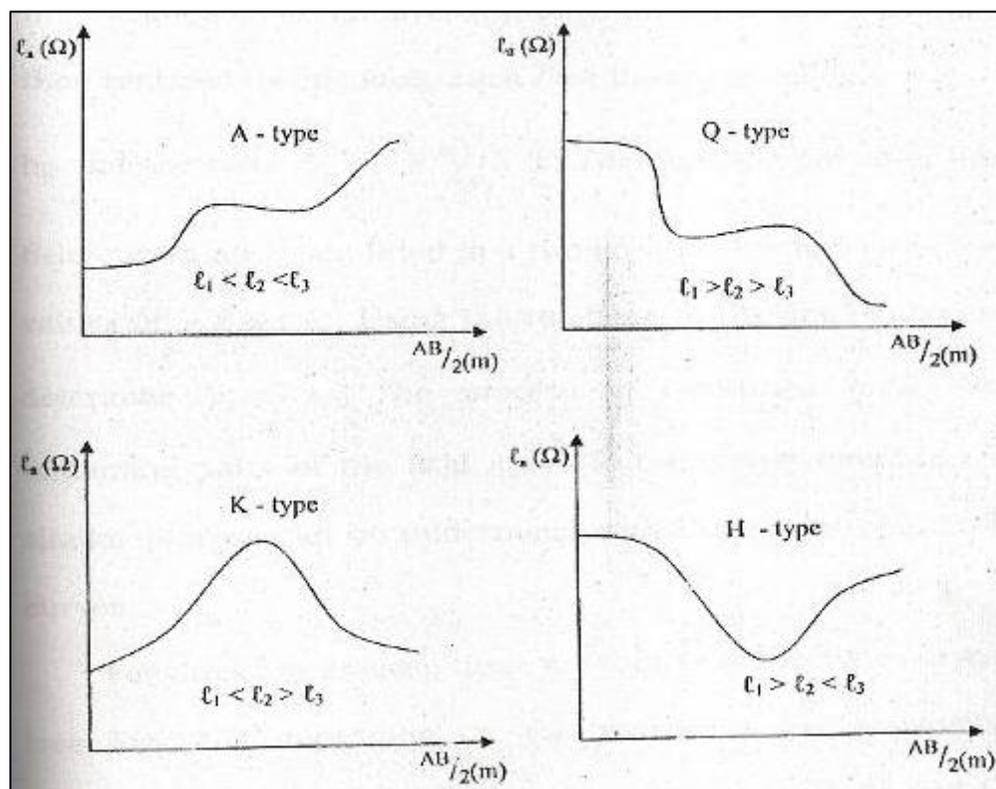
Figure 3: Typical Curves of Electrical Resistivity (VES)
