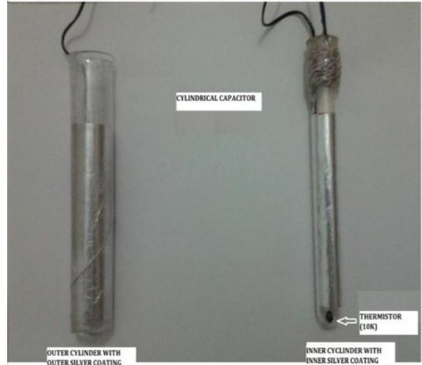
**Fig.2: Cell for Capacitance measurement with thermistor Inside the inner tube( details of size given in Ref [35])**
