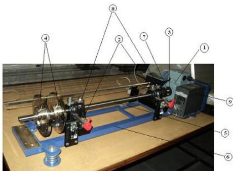
Photograph 1: Experimental setup with two rotors at overhung position
