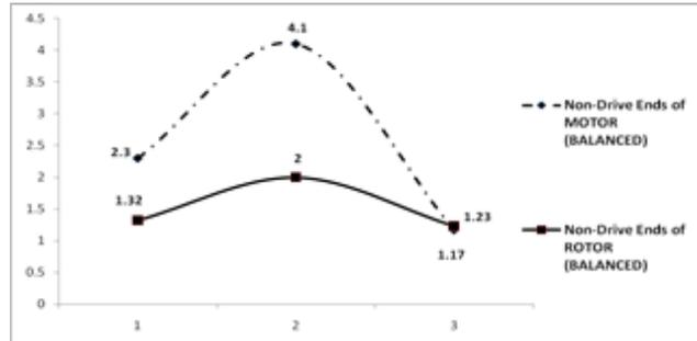
(b) Baseline Amplitude Trend of Non Drive Ends (Motor & Rotor) For 2 Rotors Overhung
