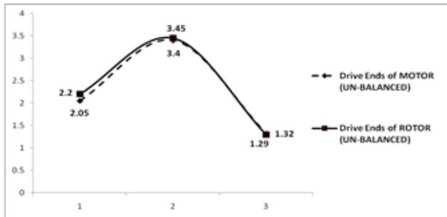
(c) Unbalanced Amplitude Trend of Drive Ends (Motor & Rotor) For 2 Rotors Overhung
