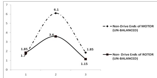
(d) Unbalanced Amplitude Trend of Non Drive Ends (Motor & Rotor) For 2 Rotors Overhung
