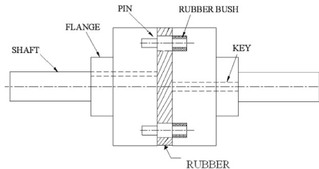
Fig.1 Four Jaw flexible coupling with key and shaft
