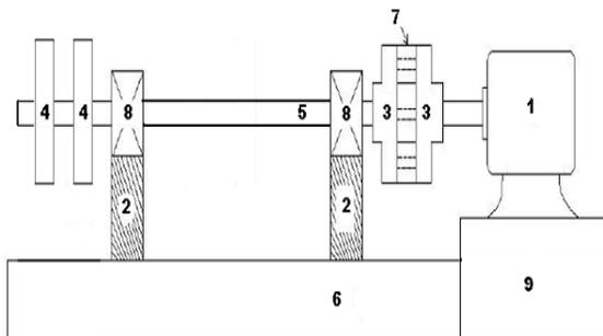
Figure 2: Experimental setup with two rotors at overhung position
