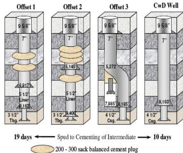
Figure 4. Casing drilling eliminates lost circulation problems [8]
