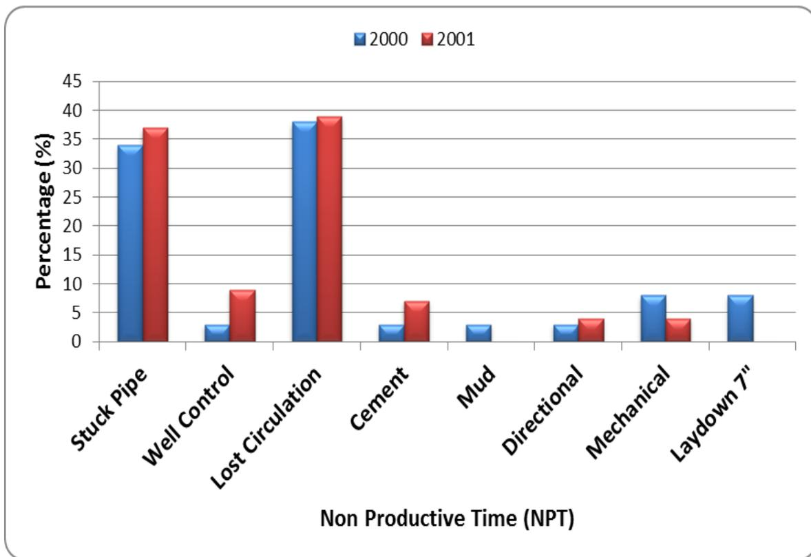
Figure 2. Trouble time for conventionally drilled well
