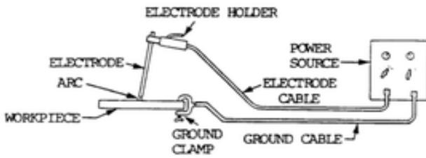
**Fig. 1: Diagram for welding setup [11].**
