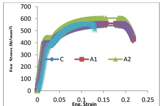
**Fig. 3: Variation of engineering stress to strain of a welded DPS**
