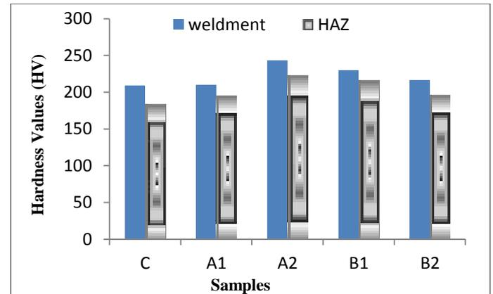
**Fig. 2: Microhardness values of welded DP steel**
