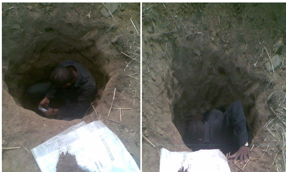
Figure 4: Trial pits for compaction analysis taken at depth of about 1.6m.
