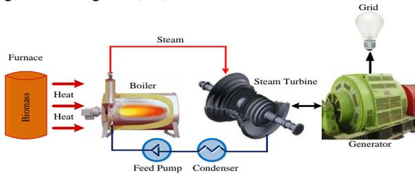
Figure 6: Flow Sheet Diagram of Conventional Steam Cycle for Power Generating
