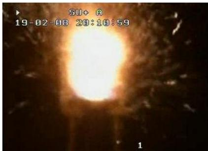
Splinters emanating from the combustor when the struts fuel injection passage is intact
