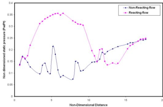
**Fig. 9 Non-Dimensional top wall static pressure distribution for the first test**
