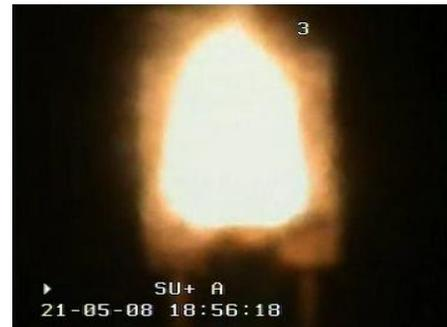
Condition of the exit plume when the strut vacuum brazed bottom blank failed
