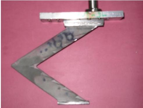
Fig.4 W-Ni-Fe alloy Strut
