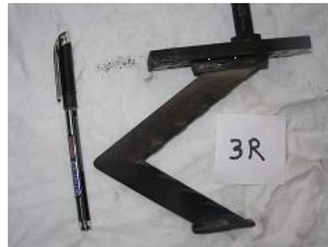
Fig.3 Niobium C-103 alloy Strut
