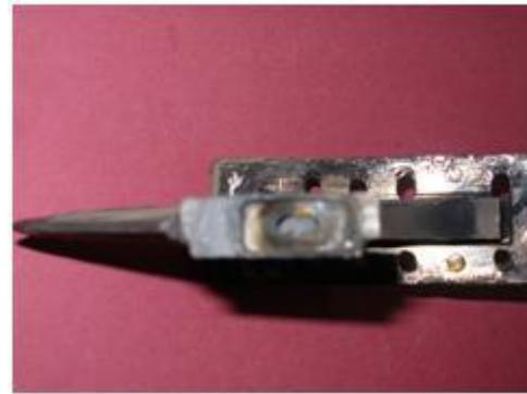
**Fig.12 Condition of the Stage-II W-Ni-Fe alloy Strut in which vacuum brazed joint failed after experiencing 20 s of supersonic combustion in the combustor**
