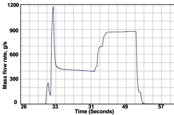
Fig.5 Mass flow rate of Kerosene in the first test
