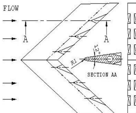
Fig.2 Schematic of fuel injection Strut
