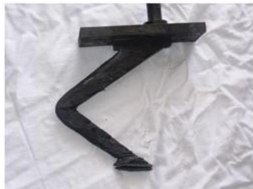
**Fig.11 Condition of the Stage-II Niobium C-103 alloy Strut after experiencing 20 s of supersonic combustion in the combustor**
