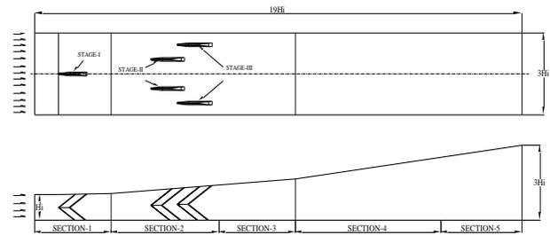
**Fig.1 Schematic of 5-Strut Scramjet combustor configuration**
