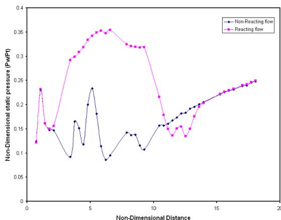
**Fig.10 Non-Dimensional top wall static pressure distribution for the second test**
