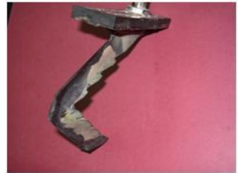
**Fig.13 Condition of the Stage-II W-Ni-Fe alloy Strut in which leading edge has eroded after experiencing 20 s of supersonic combustion in the combustor**
