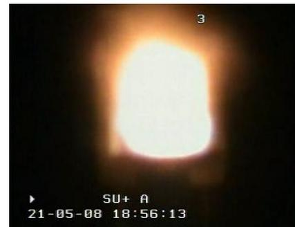
Exit plume when the struts fuel injection passage is intact
