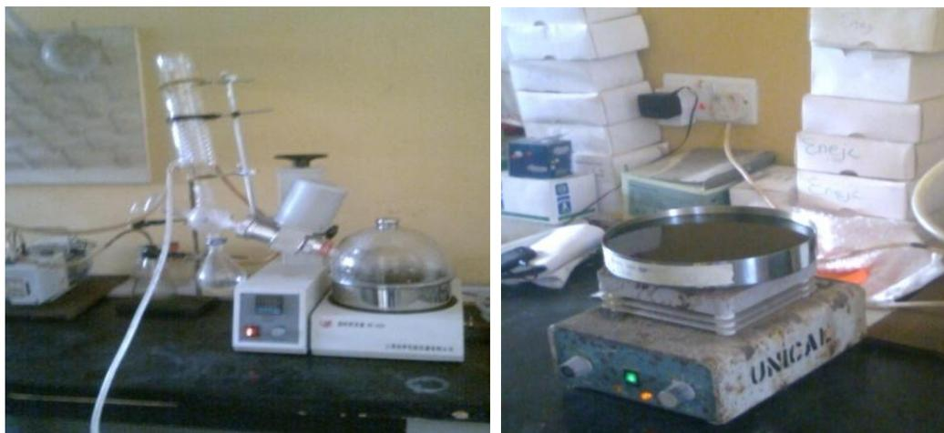
Figure 6: concentration of extracts using rotary evaporator and laboratory hot plate
