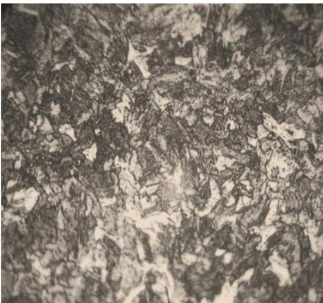
**Plate 4(a): Microstructure of Tempered (500<sup>0</sup>C) Low Carbon Steel Substrate before plating**
