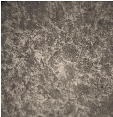
Plate 2(a): Microstructure of Quenched Low Carbon Steel Substrate before *plating*
