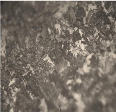
**Plate 3(a): Microstructure of Tempered (400<sup>0</sup>C) Low Carbon Steel Substrate before plating**
