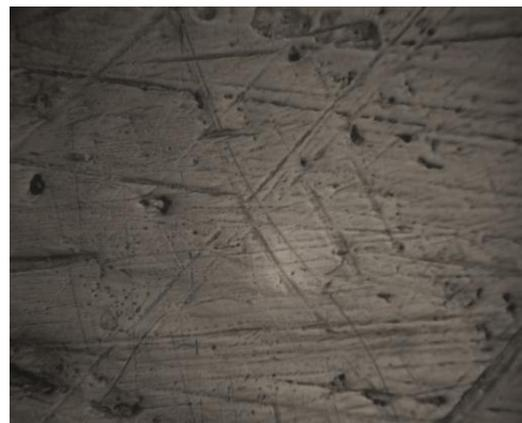
**Plate 5(b): Microstructure of Tempered (600<sup>0</sup>C) Low Carbon Steel Substrate after plating**
