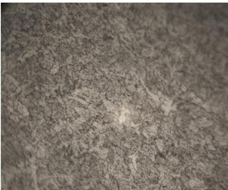
**Plate 5(a): Microstructure of Tempered (600<sup>0</sup>C) Low Carbon Steel Substrate before plating.**
