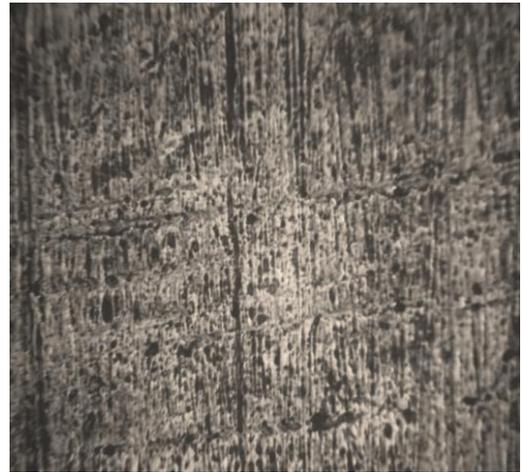
**Plate 3(b): Microstructure of Tempered (400<sup>0</sup>C) Low Carbon Steel Substrate after plating**
