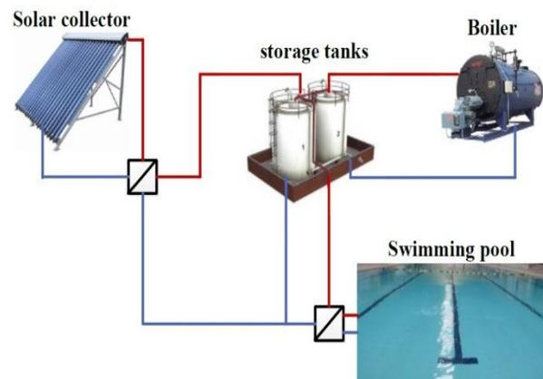
Figure 7. Scheme of the heating system for swimming pool
