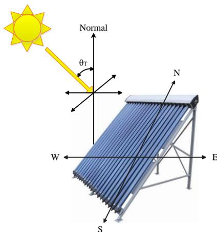
Figure 3. Measurements of the transverse incidence angle
