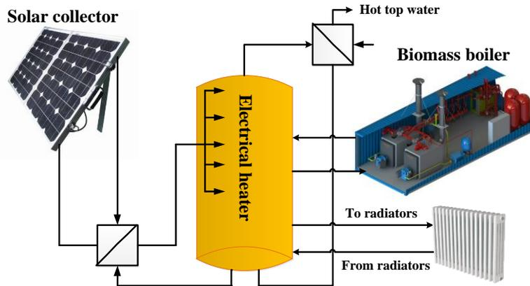
Figure 2. A solar combine system with a joint storage tank
